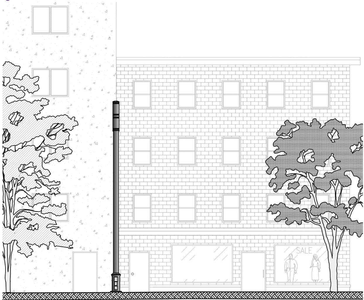
Figure 5-10: Small Cell in Commercial Area
