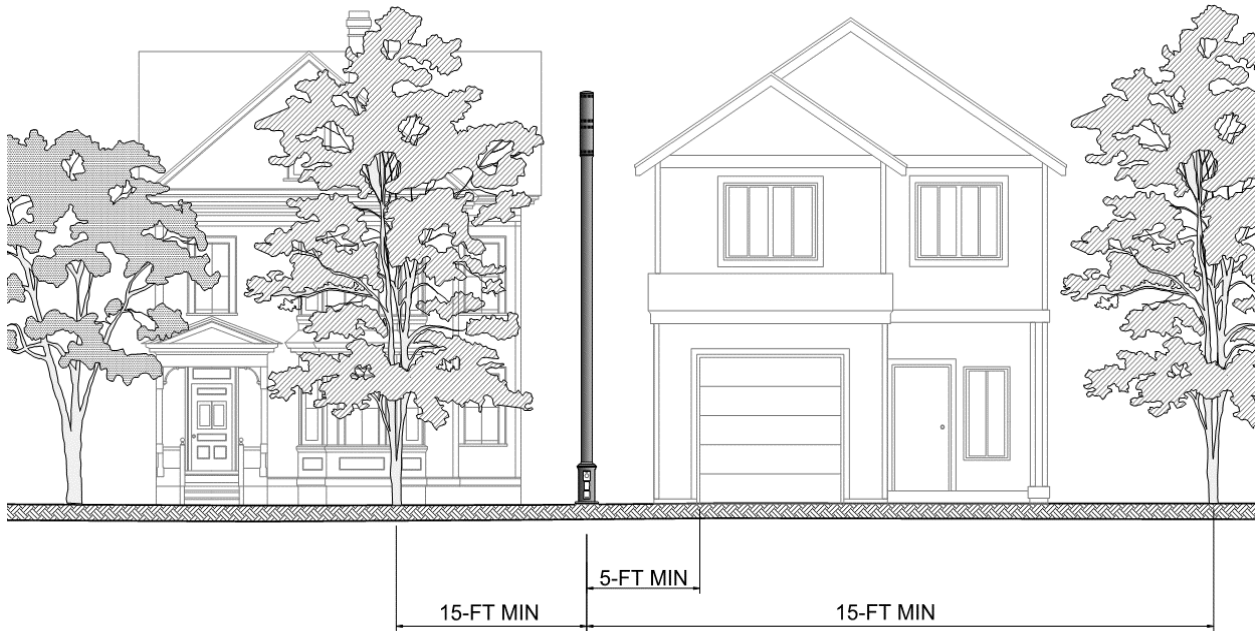
Figure 5-8: Freestanding small cell location between property and trees
