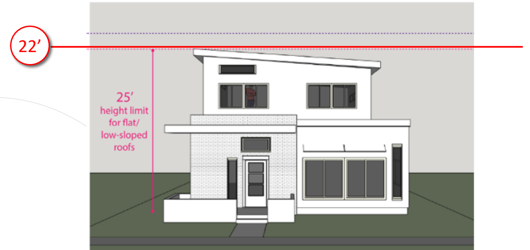
Low- Sloped Roof: 3/12 pitch or less
